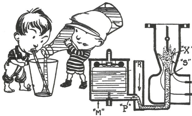
FIGURE 2—Why the compensating jet feeds at a fixed rate.
